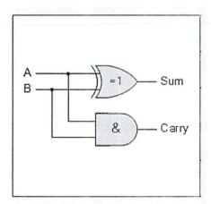
c) Draw a truth table depicting the circuit above. As shown in the diagram above your truth table should include two inputs and two outputs. Remember the output depend on the types of gate shown in the circuit. (8 Marks)
